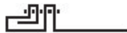
Modified running stitch of (fabric and lining, single-folded towards each other & edge of (running stitch of double-fold folded back RST)) (Fig. 55)
